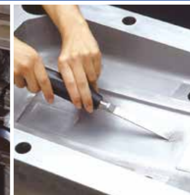
▲Wide lapping after oscillation discharge-proofing
