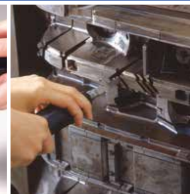
▲Deep&narrow slips (up to 180mm depth)
