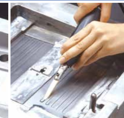
▲Mirror finish with diamond paste
